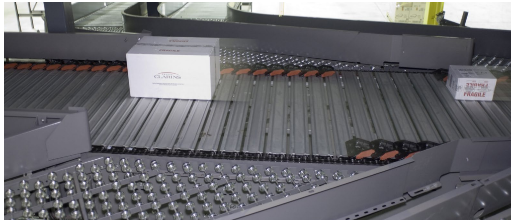
Key to throughput levels achieved by ATS in Montreal is Intelligrated's high-speed sliding shoe sorter.
